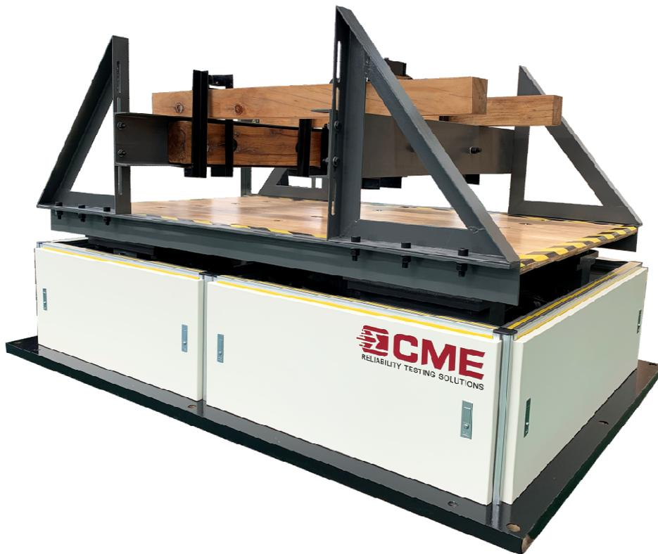
Bounce testing simulates the constant loose cargo state during truck transport. Often times, containers carrying military and civilian hardware (such as: medical supplies, electronics, weaponry, communication devices) travel for extended periods of time and must be transported off-road. All of these items must maintain functionality upon arrival at their destinations.
